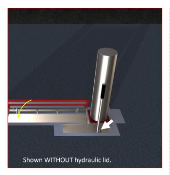
Lower the bollard cover, remove handle and LOCK the hydraulic access. Lower hydraulic lid.
