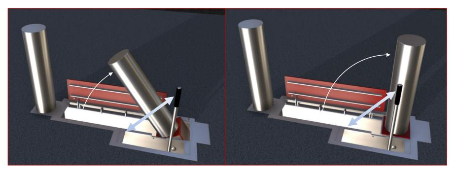
2 Continue to 'PUMP' the bollard into the fully upright position
