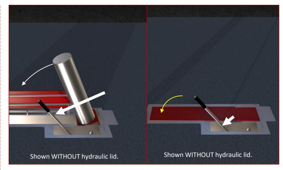
To lower. Reverse the operation and move hydraulic handle fully down to softly lower the bollard
